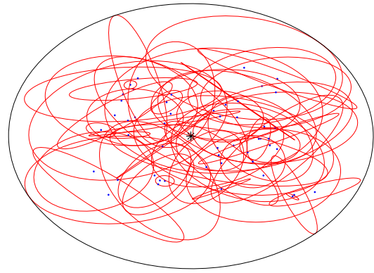
Figure 1. An approximate minimum volume ellipse containing a set of 50 randomly generated ellipses (coreset size = 4) computed using our implementation.
